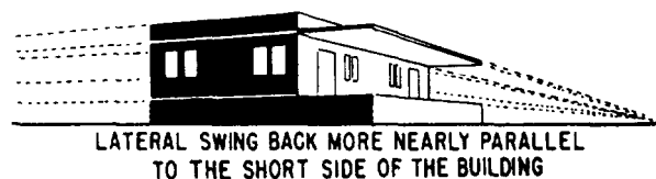
Figure 4-22.—Correction for horizontal distortion.
