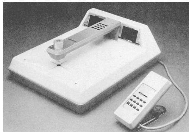
Figure 10-26.—Densitometer with both transmission and reflection capabilities.
