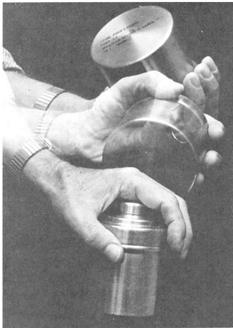
Figure 10-19.—Agitation of a small tank.
